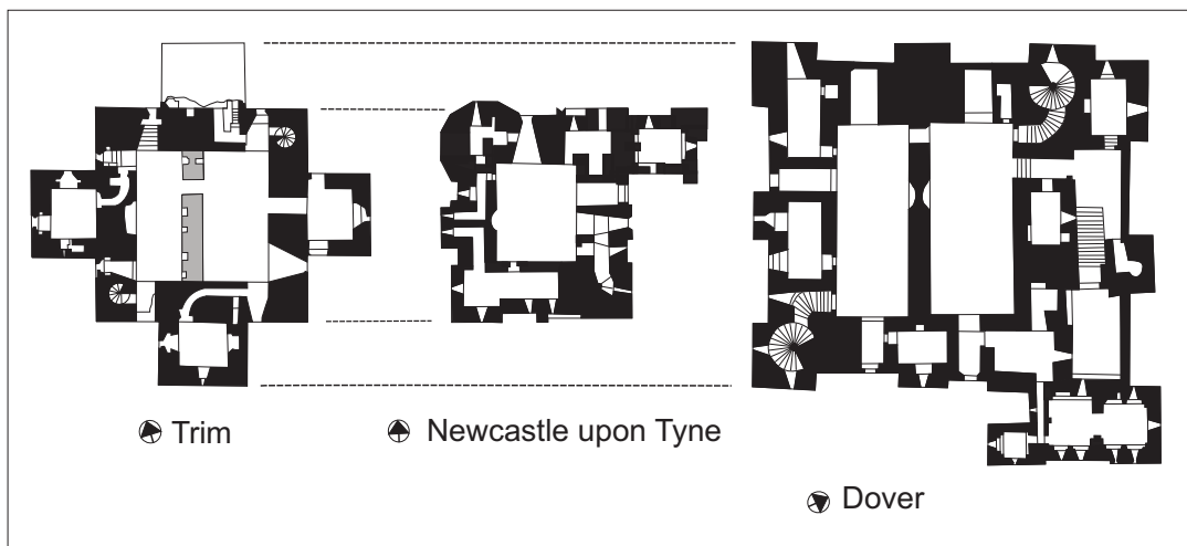
29 Plans of the donjons at Trim (first-floor level), Newcastle upon Tyne (second-floor level) and Dover (second-floor level), showing the similarities in their proportional systems.
