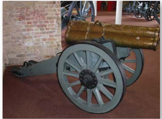
One of the anomalies of French artillery design, this light three-barrelled cannon was presumably designed for an infantry support role, firing multiple charges of canister or grapeshot into the enemy ranks at close range. (Photograph courtesy Iain Stanford)
