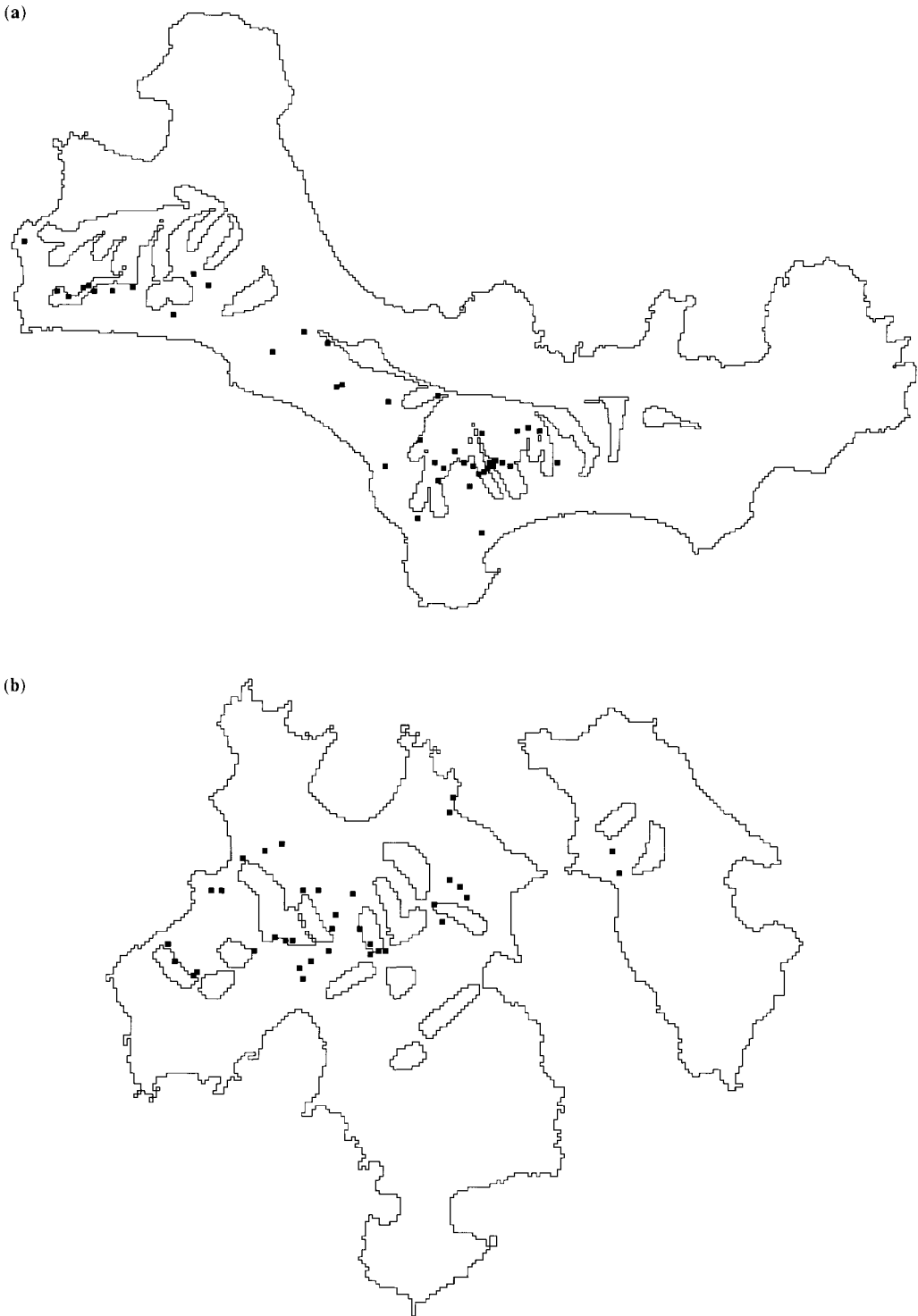
Fig. 14. Well catchment zones as derived from the results of numerical particle tracking and the positions of septic tanks. (a) St Martin's, (b) St Agnes.
